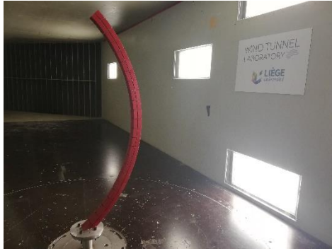
Figure 2. aeroelastic model in wind tunnel
